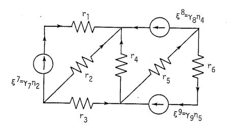
Fig.3.1. A simple electrical network of Example 3.1 (from [22])
