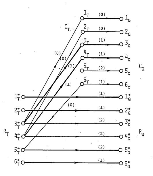
Fig. 5.1. Weighted independent-linkage problem for determining the dynamical degree of Example 4.2 (The weights are given in parentheses and the maximum-weight independent linkage is indicated by bold lines.  $I \cup J = \{1^*, 2^*, 5^*, 6^*\} \cup \{3, 4\} \text{ is a common base of } M(T_A - T_F) \text{ and } M(Q_A - Q_F).)$
